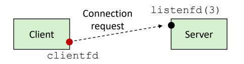
2. Client makes connection request by calling and blocking in *connect*
