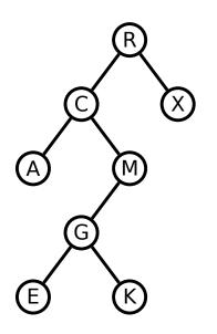
The 'P' would be inserted as the right-hand child of the 'M,' because it's before 'R,' after 'C,' and after 'M.'
