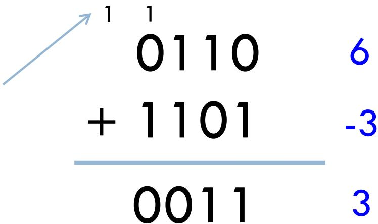
$$\begin{array}{r} 0110 \\ + 1101 \\ \hline 0011 \end{array} \quad \begin{array}{l} 1 \\ 1 \\ 6 \\ -3 \\ 3 \end{array}$$
