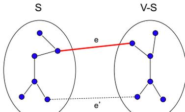
Using  $e$  instead of  $e'$ , still connects the graph, but produces a tree with smaller weights
