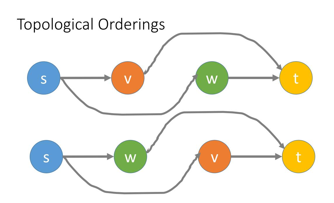
Can be used to graph a sequence of tasks while respecting all precedence constraints
