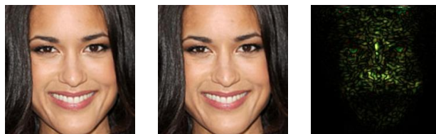
Figure 2: A dodging attack by perturbing an entire face. Left: an original image of actress Julia Jones (by Wenner Media; source: http://goo.gl/OFOIGB ). Middle: A perturbed image for dodging. Right: The applied perturbation, after multiplying the absolute value of pixels’ channels \times 20 .
